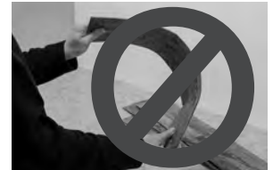
Do not bend tiles backward as it could permanently damage the tile.
