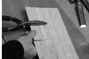
Starting a notch using a snip
